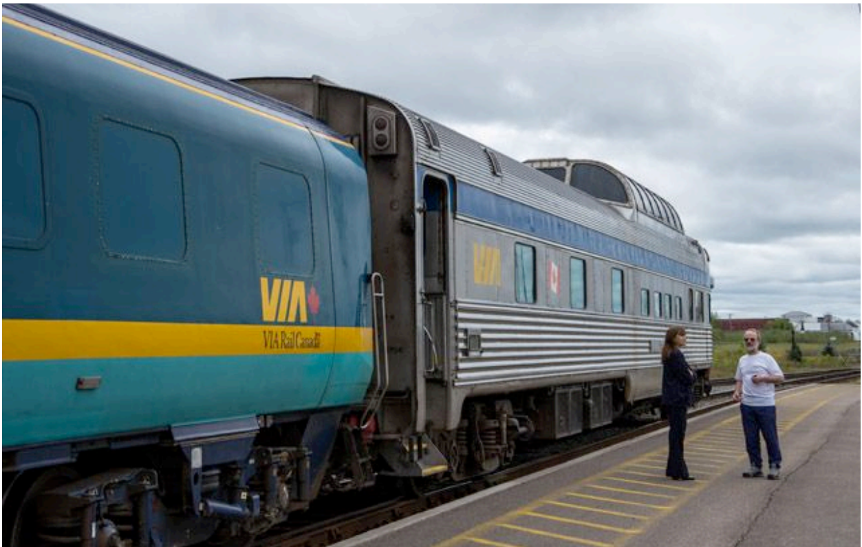
SHORT, CRAMPED AND INAPPROPRIATE: VIA's British-built Renaissance cars are expensive to operate, mechanically unreliable and ill-suited to Canadian conditions. The photo below, showing a Renaissance car (left) coupled to one of the popular and larger Budd Park cars on the Halifax-Montreal Ocean (right), demonstrates the pint-sized dimensions of this rolling stock. Photos by Steve Boyko (above) and Henry Kisor (below)
