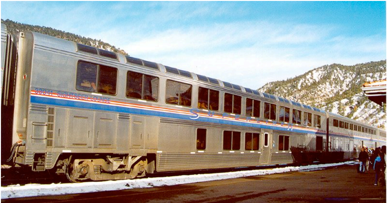
LONG-HAUL RENEWAL: Unlike VIA, Amtrak has taken numerous steps to improve the performance of its high-cost long-haul trains. The most visible example was its decision to make new rolling stock a priority. Beginning in the late 1970s, Amtrak purchased 479 bi-level Superliners for its western long-haul trains, including 195 from Canada's Bombardier Transportation. Photos by James Griffin
