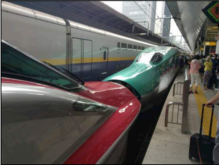
Tokyo Station, July 2013, showing new JR East high speed trains. Green E5 is a 10-car set coupled to a red E6 7-car set used in northern Shinkansen service. Top speed is 320 kph. Train sets are capable of operating in winter weather. Behind is an E4 bi-level train set. Two coupled 8-car E4 train sets have 1,634 seats, the highest capacity high speed trains in the world. Top speed is 240 kph. Photo: Kyle Woodmansey.
