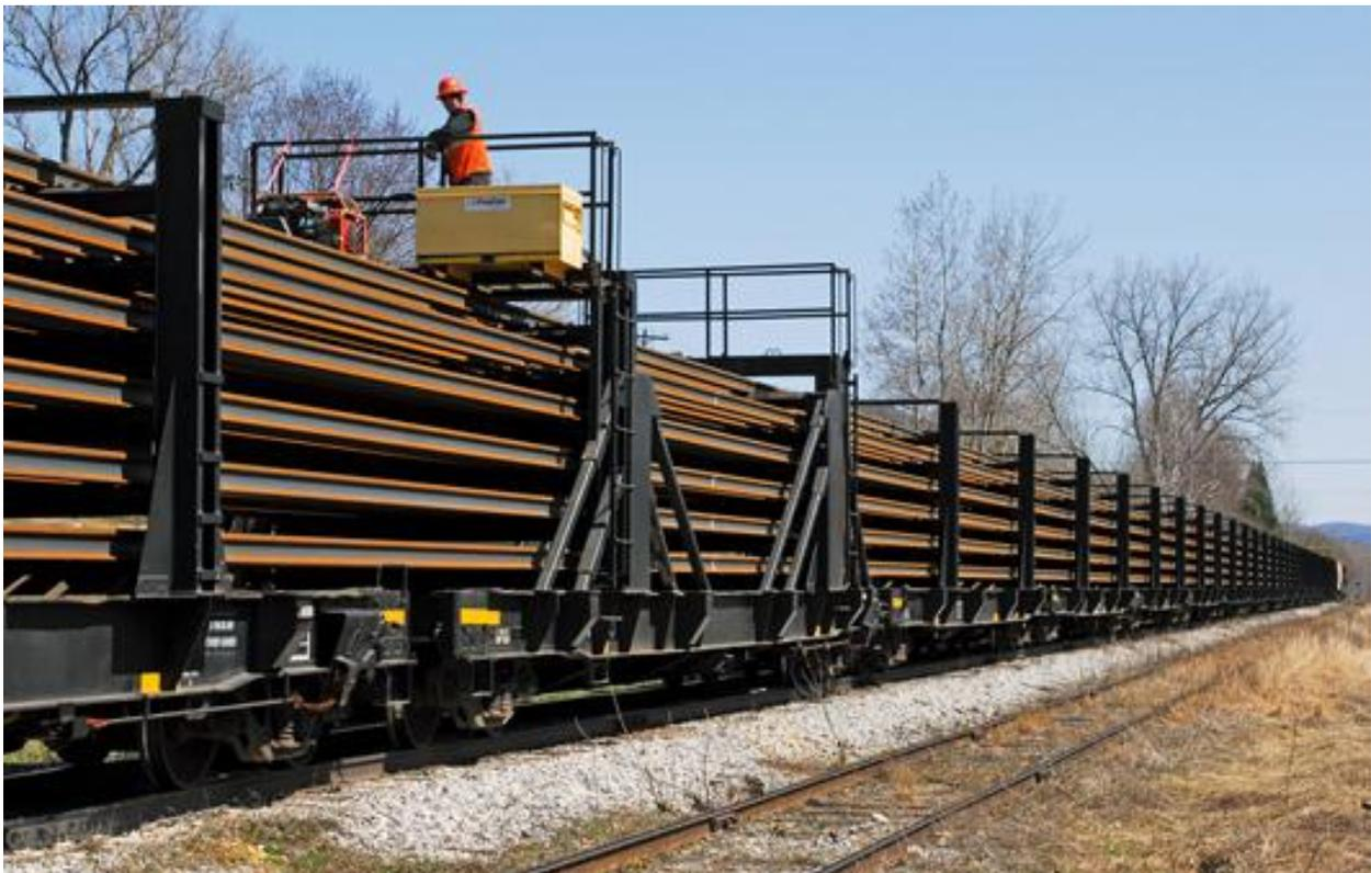
**RENEW IT OR LOSE IT:** The Newcastle Subdivision cannot survive for long in its present condition. The line must be renewed soon, especially the 60-mile section between Rogersville and Bathurst, which desperately needs new continuous welded rail (shown above), new ties, deeper ballast and bridge repairs. Whether under CN or public ownership, the public's interest and investment must be fully protected to prevent a repeat of the current CN abandonment threat.
