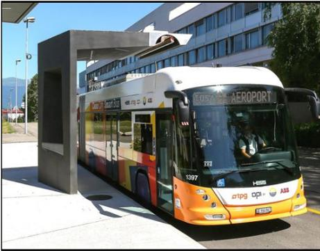
Experimental flash charged electric bus taking on power at an overhead charging facility in Geneva, Switzerland. Image: EPFL, 2014.
