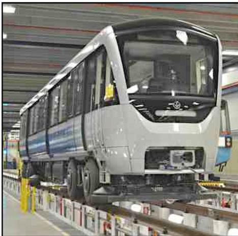
Société de transport de Montréal's new Azur subway car was unveiled April 28. First ordered in 2010, Bombardier/Alstom are jointly building 468 cars for 52 nine-car trains. Trains feature a full-width walkway; top speed is 72.4 kph. The cars have rubber-tire trucks, first developed for selected lines of the Paris metro. Montreal's subway opened in 1966.
